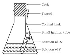
**Fig. 3.1:** Ignition tube containing solution of X, dipped in a conical flask containing solution of Y.
